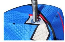
The chimney section is made of stainless steel and special fiberglass with a silicone double sided coating, designed for stove with 90 mm chimney diameter. To install stove with a smaller diameter of the chimney, it is recommended to use an adapter ring. There is a ventilation window for the air to reach the stove. The window has a mosquito net.
